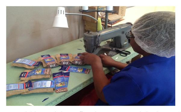
Figure 44: Labels being stitched on to coffee packages at Jamaica Standard Products Limited
